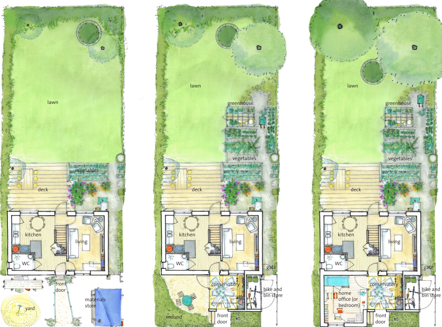
Phase 1a A highly insulated, near-passivhaus standard 69 sqm two-storey house core with kitchen, living and two bedrooms that can be built for £43,460.
