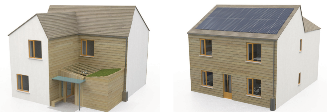
Alternatively, the roof and front face of the house could be clad with cedar shingles, with the sides and back of the house rendered, and timber windows clear finished. The house is shown at the end of Phase 2.
