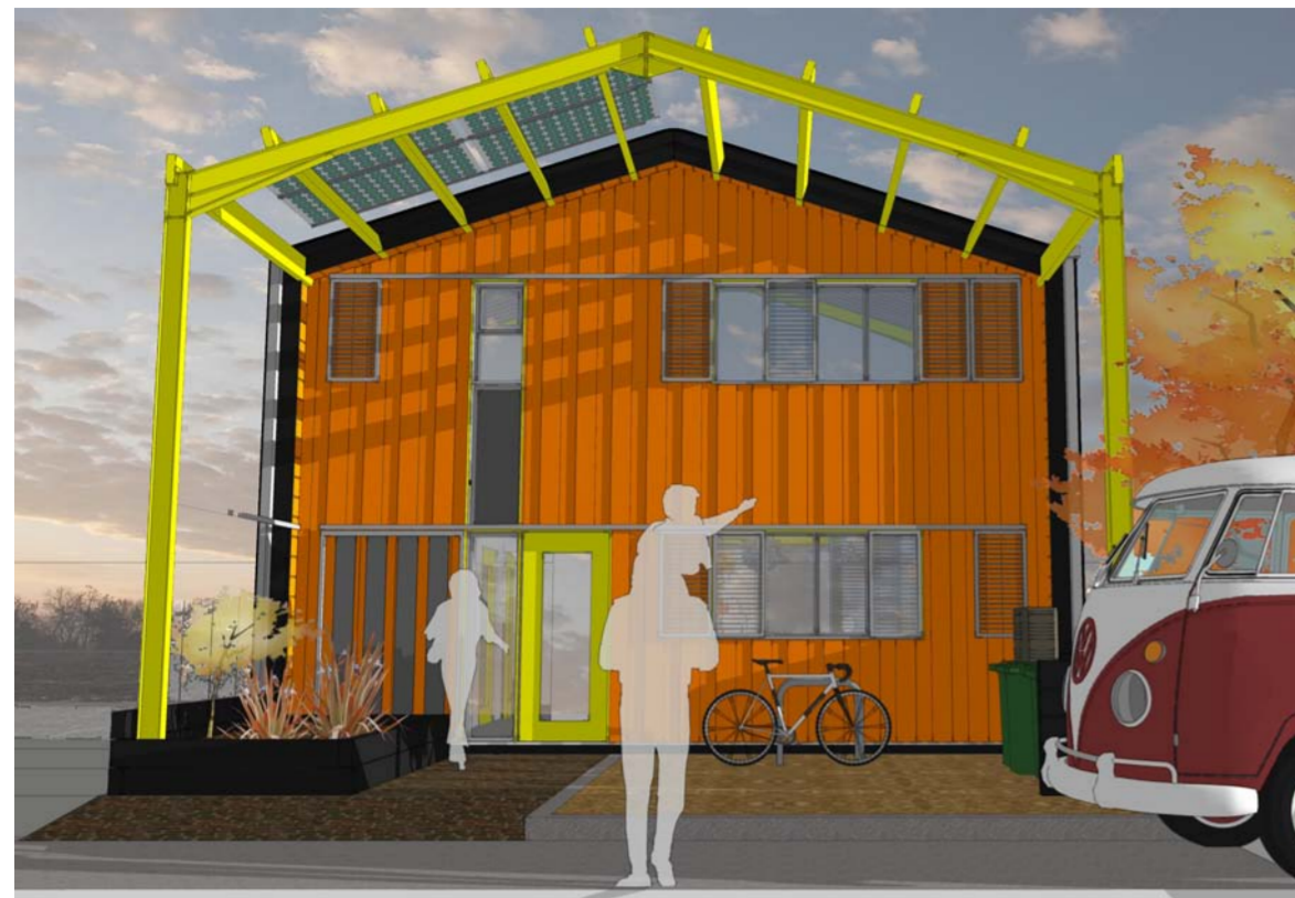
STREET VIEW - North elevation shows planting, shuttered windows and PV canopy
